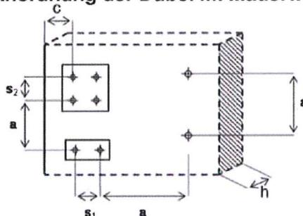
$$a \geq \max(250 \text{ mm}; s_{1,min}; s_{2,min})$$
